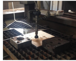
b. Water jet cutting experiment site
