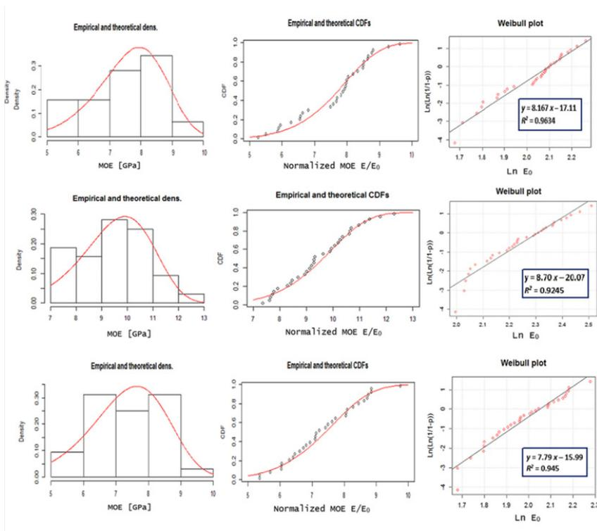
Fig. 4: The probability density function, the cumulative distribution function and the Weibull plot for the L0° (top), the L45° (middle), and the L90° orientation (down).
