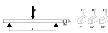
Fig. 2: Tree-point bending test arrangement and direction of load in relation to annual growth ring orientation.
