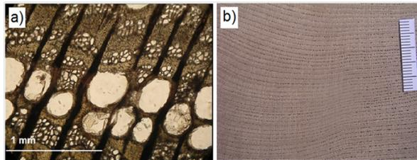
Fig. 1: Micro (a) and macro (b) cross section of the sample (*Ulmus minor*).
