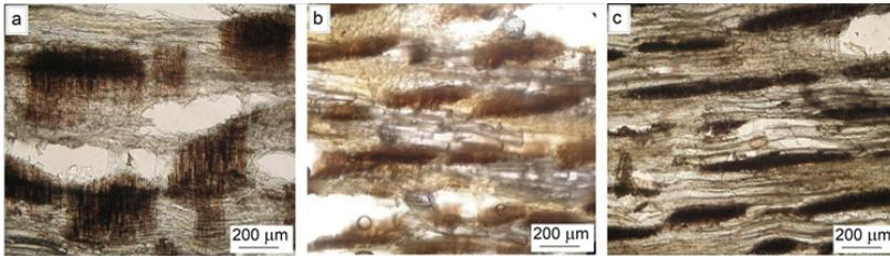
Fig. 3: Microstructure of longitudinal section at three annual growth ring orientations:  $L0^\circ$  (a),  $L45^\circ$  (b) and  $L90^\circ$  (c).
