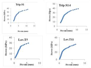
Fig. 2: Strain-Stress curves for bending tests on Triplochiton scleroxylon (Trip.s) and Lovoa trichilioides (Lov.t)
