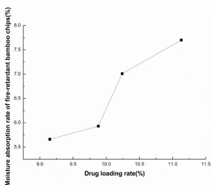
Fig. 6: Effect of drug loading rate on water absorption rate of fire retardant bamboo chips.
