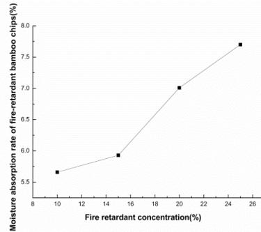
Fig. 2: Effect of fire retardant concentration on water absorption rate of fire retardant bamboo chips.
