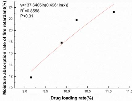
Fig. 3: Correlation analysis of drug loading rate and water absorption rate of fire retardant.
