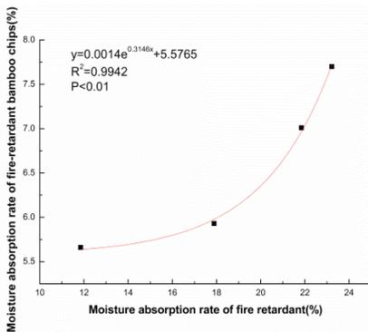
Fig. 7: Correlation analysis of water absorption rate on fire retardant and fire retardant bamboo chips.
