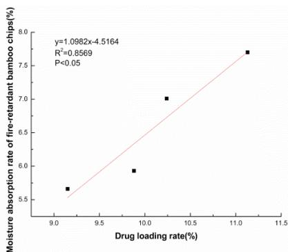
Fig. 5: Correlation analysis of drug loading rate and water absorption rate of fire retardant bamboo chips.
