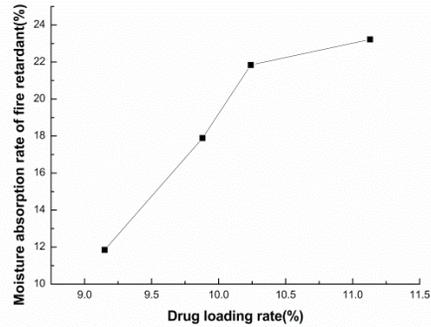
Fig.4: Effect of drug loading rate on water absorption rate of fire retardant.
