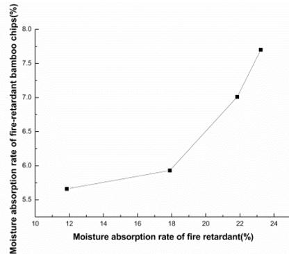
Fig. 8: Effect of water absorption rate of fire retardant on the water absorption rate of fire retardant bamboo.
