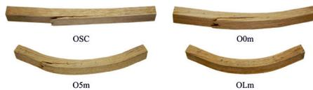
Fig. 6: Images of crack patterns for different modification methods. Abbreviations: OSC-steamed control sample; O0m, O5m-longitudinally compressed samples with 0 and 5 minutes of relaxation time; OLm-compressed and a long-time relaxed sample.
