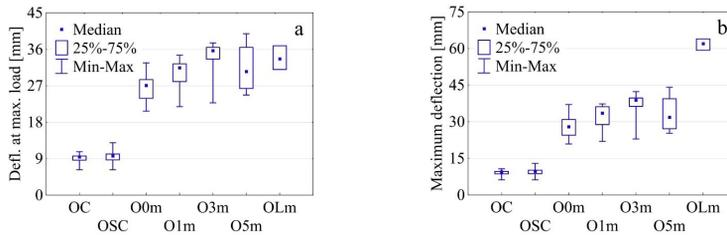
Fig. 4: The deflections at the highest bending forces (a), and the maximum deflections (b) during 4 point bending test. Abbreviations: OC-control sample; OSC-steamed control sample; O0m, O1m, O3m, O5m-longitudinally compressed samples with 0, 1, 3 and 5 minutes of relaxation time; OLm-compressed and long-time relaxed sample.
