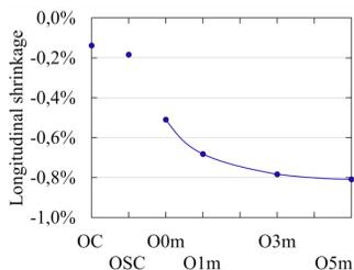
Fig. 7: Length change during the drying process, depending on the relaxation time. Abbreviations: OC-control sample; OSC-steamed control sample; O0m, O1m, O3m, O5m-longitudinally compressed samples with 0, 1, 3 and 5 minutes of relaxation time.
