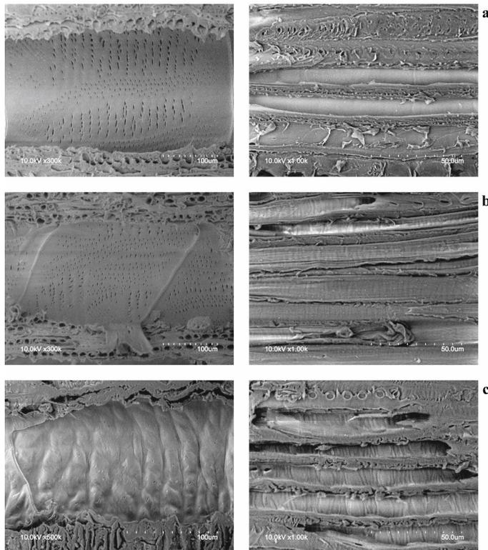
Fig. 2: Scanning electron microscopy images of the trachea (left; 10 kV x300 and x500) and the fibres (right; 10 kV x1000) of oak wood in a control sample (a), a longitudinally compressed sample without relaxation (b), and a longitudinally compressed sample with long-time relaxation (c).
