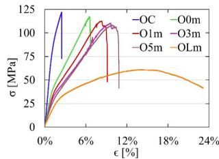
Fig. 5: Typical Relative deformation – Bending stress graphs for the different treatments. Abbreviations: OC-control sample; O0m, O1m, O3m, O5m-longitudinally compressed samples with 0, 1, 3 and 5 minutes of relaxation time; OLm-compressed and long-time relaxed sample.
