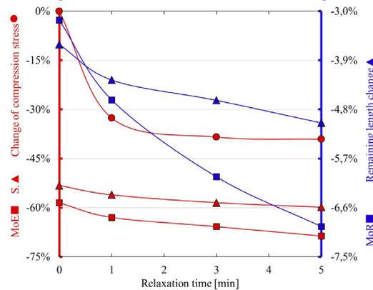
Fig. 3: Mechanical and physical properties after compression with the increasing relaxation time. Abbreviations: S–Stress change at 5 mm load span displacement; MoE–change of modulus of elasticity; MoR–change of modulus of rupture.
