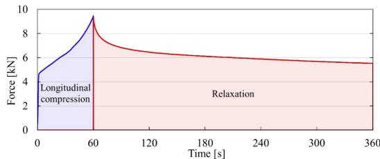
Fig. 1: A typical Time - Force graph of a longitudinal compression with a 5 minute relaxation.
