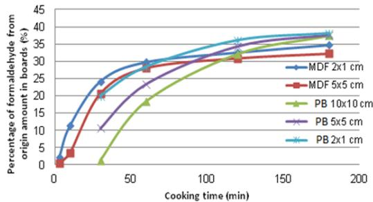
Fig. 1: Resin hydrolysis of waste MDF and PB depending on sample size and cooking time.
