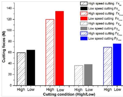
Fig. 4: The influence of cutting speed on cutting forces (cutting length=0m).
