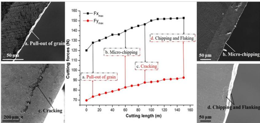
Fig. 8: The influence of maximum cutting forces and cutting length on abnormal wear shown on the micrographs of tool wear at high speed cutting.
