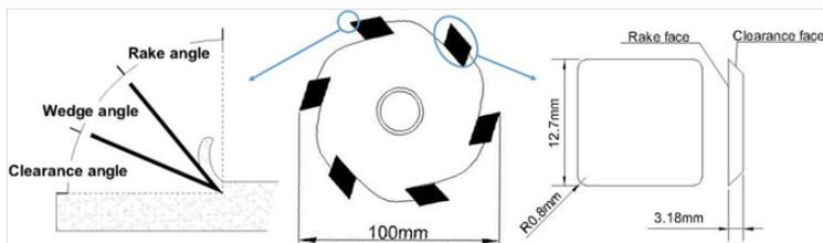
Fig. 1: The model figure of ceramic cutting tools.
