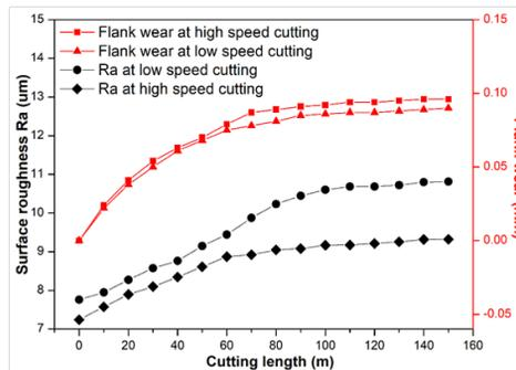
Fig. 11: The influence of the cutting length on the tool wear and surface roughness (machining quality) at high speed cutting.
