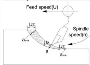
Fig. 2: The model of cutting parameters .
