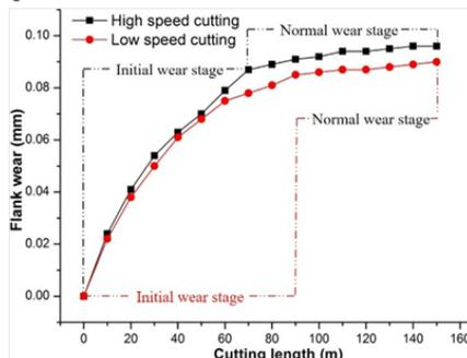
Fig.6: The influence of cutting length and cutting speed on flank wear.
