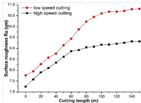
Fig. 7: The influence of cutting length and cutting speed on surface roughness as a machining quality.
