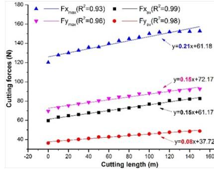
Fig. 5: The influence of cutting length on cutting forces.
