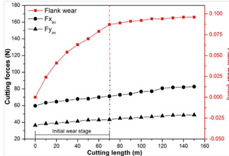
Fig. 10: The influence of cutting length on cutting forces and the flank wear (machining quality) at high speed cutting.
