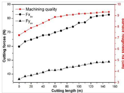
Fig. 9: The influence of cutting length on the cutting forces and surface roughness (machining quality) at high speed cutting.
