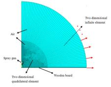
Fig. 5: Finite element model after meshing.
