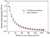
Fig. 9: Electric field intensity distribution under the electrostatic spray gun.
