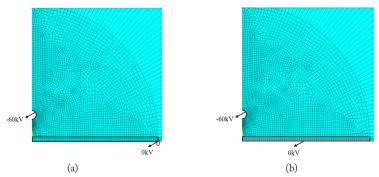
Fig. 6: Boundary conditions of two electrostatic spraying methods. (a) Traditional method, (b) New method.
