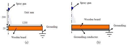
Fig. 4: Simulation models of two electrostatic spraying methods. (a)Traditional electrostatic spraying method, (b) New electrostatic spraying method.
