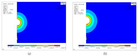
Fig. 8: Electric field intensity of two electrostatic spraying methods. (a) Electric field of traditional method, (b) Electric field of the new method
