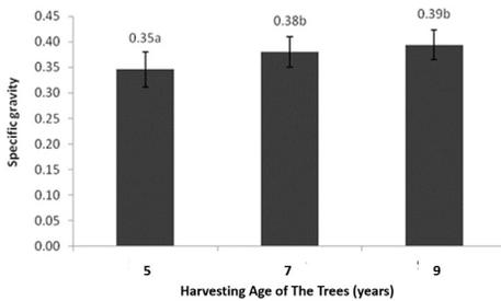
Fig. 2: The Average specific gravity of *Paraserianthes falcataria* wood from three different rotation age of tree.
