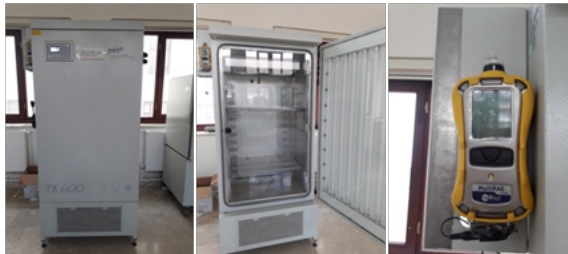
Fig. 1: Climatic test cabinet and multi-RAE multiple gas analyzer.
