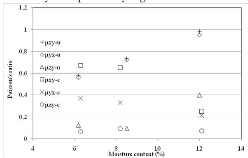
Fig. 5: Moisture dependent Poisson's ratios of face layers determined by ultrasound (u) and compression (c) tests.
