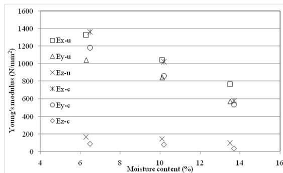
Fig. 2: Moisture dependent Young's modulus of core layers determined by ultrasound (u) and compression (c) tests.
