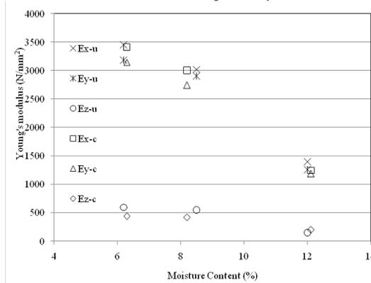
Fig. 1: Moisture dependent Young's modulus of face layers determined by ultrasound (u) and compression (c) tests.
