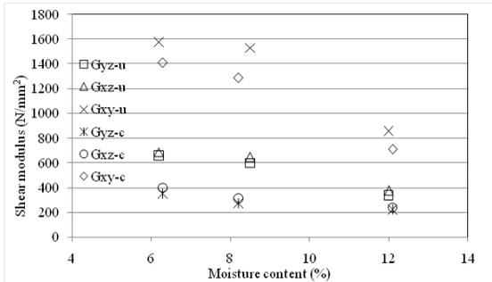
Fig. 3: Moisture dependent shear modulus of face layers determined by ultrasound (u) and compression (c) tests.
