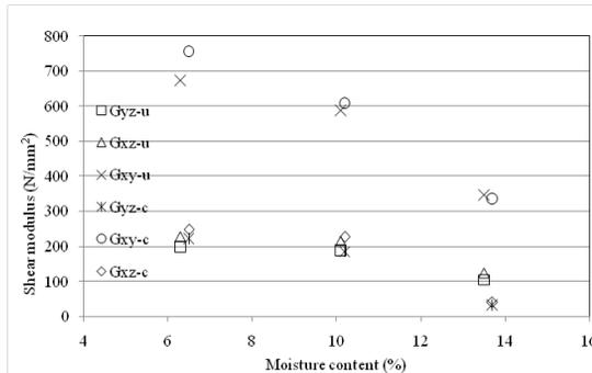
Fig. 4: Moisture dependent shear modulus of core layers determined by ultrasound (u) and compression (c) tests.
