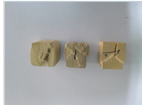
Fig.4: Compression failure modes in the grain direction.
