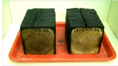
Fig. 5: Charred stud specimens after heat exposure experiments.
