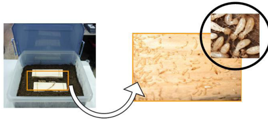
Fig. 1: Example of testing colony: detail of wooden slats infested with termites.
