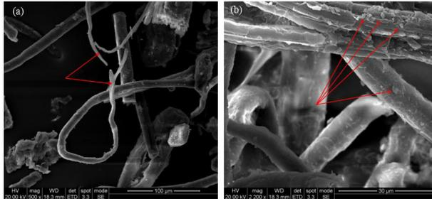
Fig. 3: The surface morphology of bamboo after steam explosion. (a) 500X. (b) 2200X.
