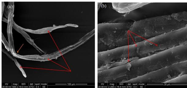
Fig. 2: The surface morphology of poplar after steam explosion. (a) 500X. (b) 2200X.
