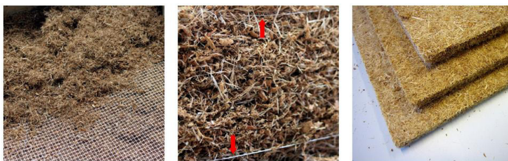
Fig. 1: Preparation of panels with mesh sheets (red arrows) and the manufactured panels.
