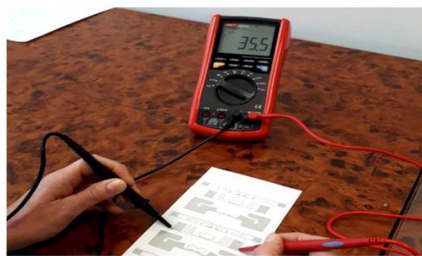
Fig. 5: Measurement of electrical resistance of UHF RFID antennas with UNIT-T multimeter, model UT70B.
