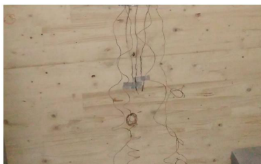
Fig. 6: Unexposed side of the test sample after the medium-scale test.
