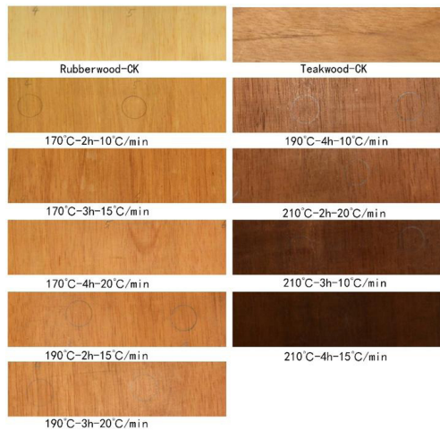
Fig. 5: Control wood samples (rubber wood and teak wood) and heat-treated rubber wood.
