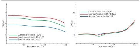
Fig. 6: TG–DTA analysis on nifa frond particleboards at pressing temperature 200°C and various ratio sucrose/citric acid.
