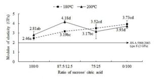
Fig. 3: Modulus of elasticity (MOE) of nipa frond particleboards on various pressing temperatures and ratio of sucrose/citric acid. Error bars indicate standard deviation. Mean values followed by different letters indicate that are significantly different (p < 0.05).
