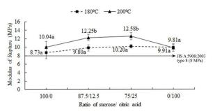
Fig. 2: Modulus of rupture (MOR) of nipa frond particleboards on various pressing temperatures and ratio of sucrose/citric acid. Error bars indicate standard deviation. Mean values followed by different letters indicate that are significantly different (p < 0.05).
