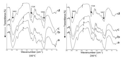
Fig. 4: FTIR analysis pressing temperatures 180°C and 200°C, and ratio of sucrose/citric acid 100/0 (a), 87.5/12.5 (b), 75/25 (c), and 0/100 (d).
