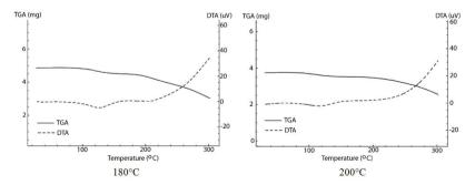
Fig. 5: TG-DTA analysis on nipa frond particleboards at ratio sucrose/citric acid 0/100 and various pressing temperatures.
