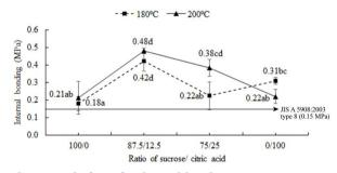
Fig. 1: Internal bonding strength of nipa frond particleboards on various pressing temperatures and ratio of sucrose/citric acid. Error bars indicate standard deviation. Mean values followed by different letters indicate that are significantly different (p < 0.05).
