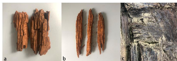
Fig. 1: Two types of decayed wood of coffin (a, b) and wooden slips (c).
