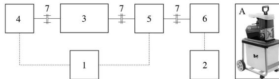
Fig. 1: Scheme of the test stand: 1 – recording computer, 2 – wood chipper controller, 3 – working unit, 4 – RPM sensor, 5 – torque measurement device, 6 – drive motor, 7 – clutch; detail A shows the cylinder wood chipper before fitting the measurement devices.
