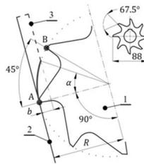
Fig. 5. Geometry of comminution process with a single cylinder wood chipper, where: 1 – grinding cutter, 2 – pressure plate, 3 – material under comminution,  $L$  – length of surface under comminution,  $b$  – thickness of material under comminution,  $R$  – blade radius of the mill,  $\alpha$  – theoretical angle required for cutting the material through,  $A$  – vertex of the first blade,  $B$  – vertex of the second blade.
