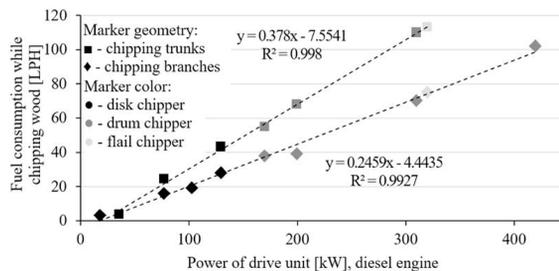
Fig. 6. Fuel consumption of heavy duty, self-ignition engined industrial wood chipper (elaborated basing upon results of investigations (Facello et al. 2013, Manzone 2015, Shahid et al. 2019).
