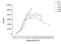
Fig. 8: Compared load-displacement curves of interlaminar shear test.
