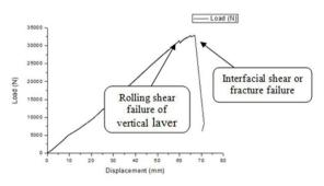
Fig. 3: Load-displacement curve of CLT in four-point bending test.
