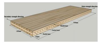
Fig. 1: Three layers CLT structure diagram.
