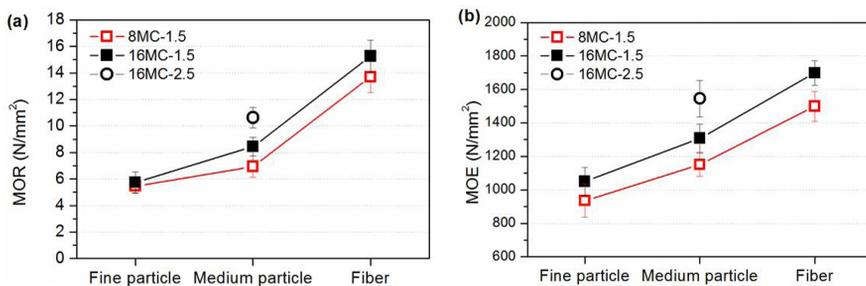
Fig. 5: MOR (a) and MOE (b) values of 15 mm particleboard. Note: the sample code refers to Tab. 1.
