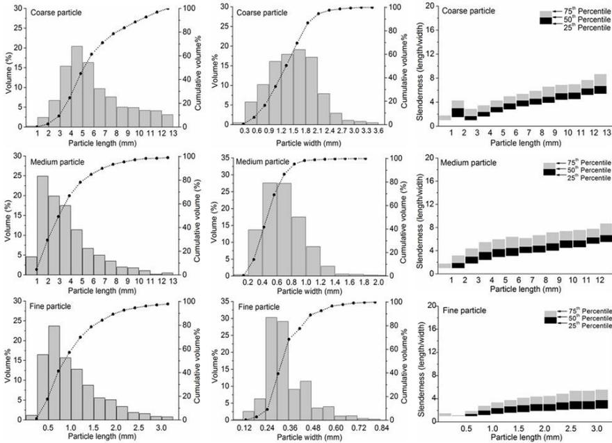
Fig. 2: Histogram of the distribution and cumulative distribution of the particle length and width, and Box plot of particle slenderness.
