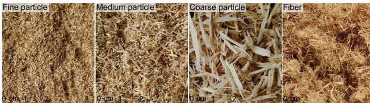
Fig. 1: Wood particle and fiber used for manufacturing of low density particleboard.
