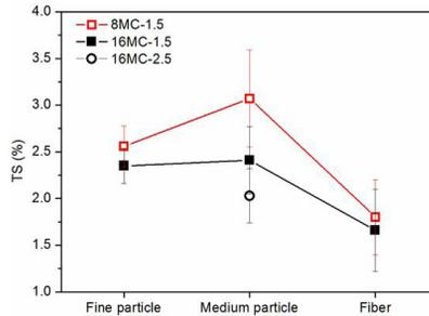
Fig. 7: Thickness swelling (TS) of particleboards after 2 h water soaking.
