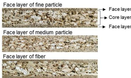
Fig. 3: Internal structure of 15 mm three-layer particleboards with 1.5 mm face layer made from fine particle, medium particle and fiber, respectively.
