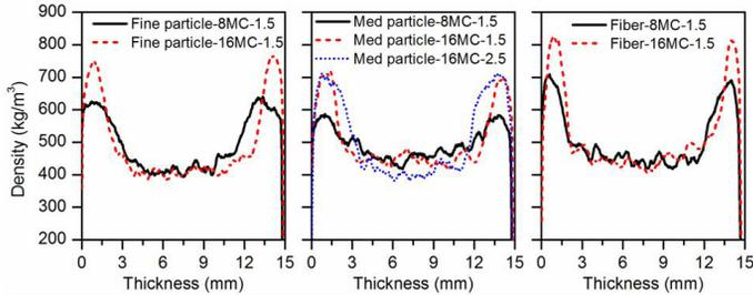
Fig. 4: Vertical density profiles of particleboards with different formulations. The sample code refers to Tab. 1.
