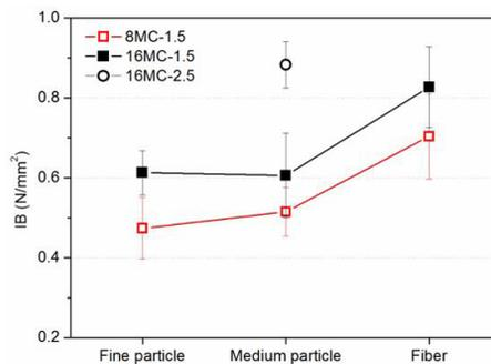
Fig. 6: Internal bond strength of 15 mm low density particleboard with different face layer material and MC. Note: the sample code refers to Tab. 1.
