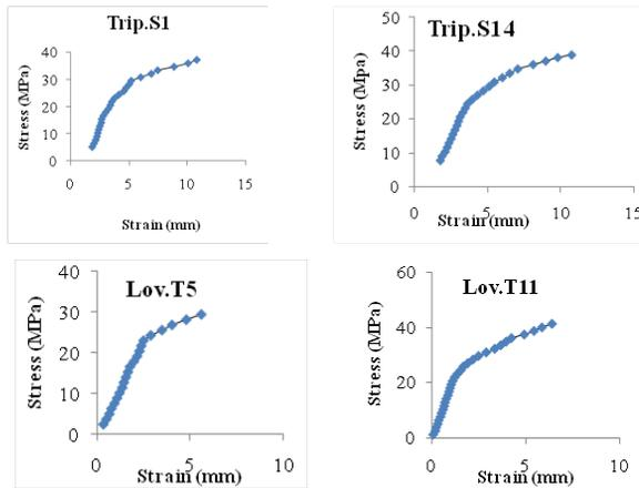
Fig. 2: Strain-Stress curves for bending tests on *Triplochiton scleroxylon* (*Trip.s*) and *Lovoa trichilioides* (*Lov.t*)
