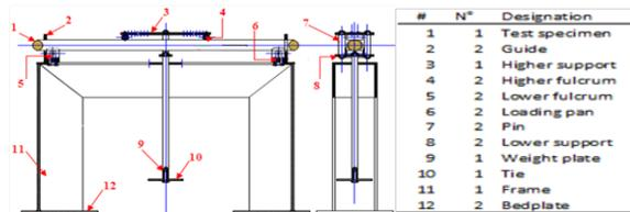
Fig. 1: Bending test device (Talla and Foadieng 2010).
