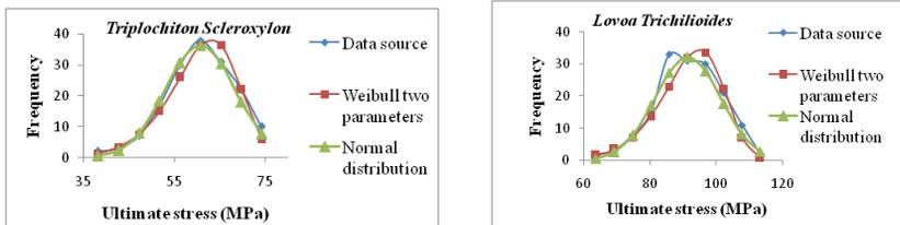
Fig. 4: Comparison of data, Weibull 2-parameter and the normal distributions.
