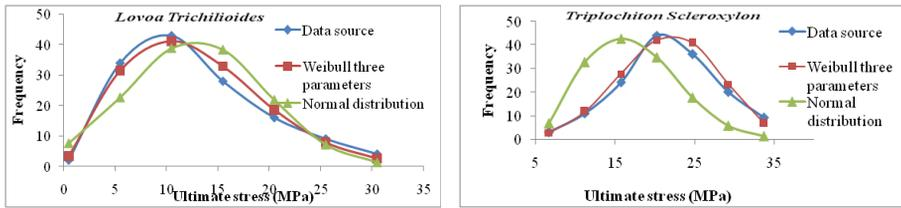
Fig. 6: Comparison of experimental data, three-parameter Weibull distribution and normal distribution.
