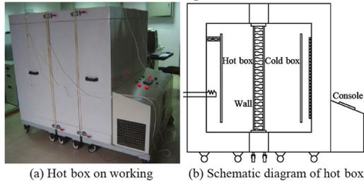
Fig. 3: The structure of hot box.
