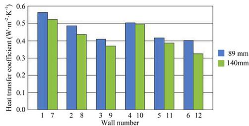
Fig. 7: Effect of studs thickness on heat transfer coefficient.
