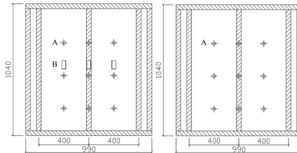
Fig. 4: The schematic diagram of measuring points. (A is T-type thermocouple; B is heat flow meter.)
