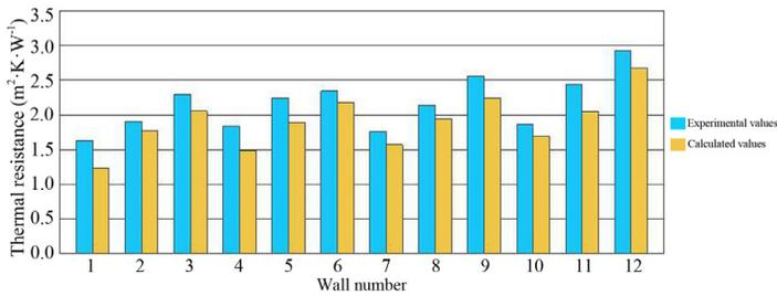
Fig. 8: Contrast of experimental and theoretical calculation.
