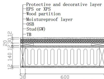
Fig. 2: The wall frame structure.
