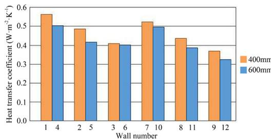
Fig. 6: Effect of stud spacing on heat transfer coefficient.
