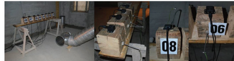
Fig. 4: Samples in sanitized area with the Acoustic Pack system sensors and with thermoelectric sensors.
