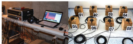
Fig. 7: Sensors S1 - S8 on wood samples and the Acoustic Pack system in the process of measuring (Čeladná, the district of Frýdek - Místek, Czech Republic).
