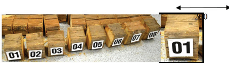
Fig. 1: Cut-outs of test samples before infecting with the detail of width measurement in the fibre direction.
