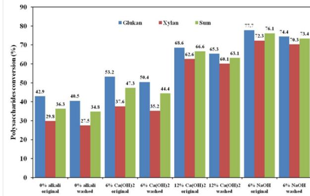
Fig. 2: Effect of NaOH and Ca(OH)<sub>2</sub> loading in extrusion pretreatment on polysaccharides conversion of original and washed extruded wheat straw after 72 h of enzymatic hydrolysis.
