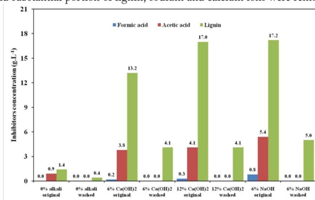
Fig. 4: Effect of NaOH and  $\text{Ca}(\text{OH})_2$  loading in extrusion pretreatment on concentration of formic acid, acetic acid and lignin in hydrolysates of original and washed extruded wheat straw after 72 h of enzymatic hydrolysis.
