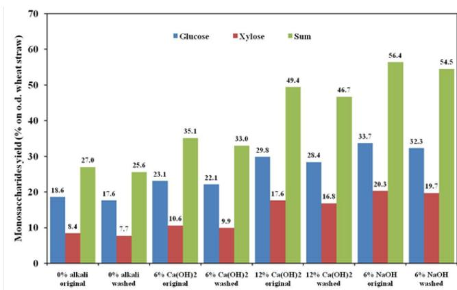
Fig. 3: Effect of NaOH and Ca(OH)<sub>2</sub> loading in extrusion pretreatment on monosaccharides yield of original and washed extruded wheat straw after 72 h of enzymatic hydrolysis.
