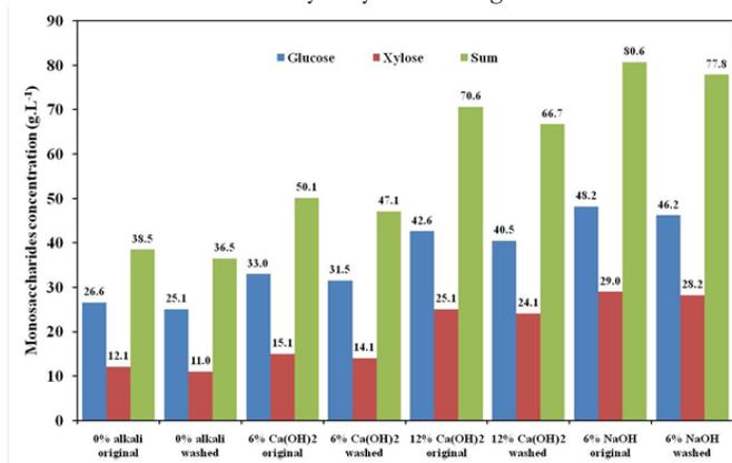
Fig. 1: Effect of NaOH and Ca(OH)<sub>2</sub> loading in extrusion pretreatment on monosaccharides concentration in hydrolysates of original and washed extruded wheat straw after 72 h of enzymatic hydrolysis.
