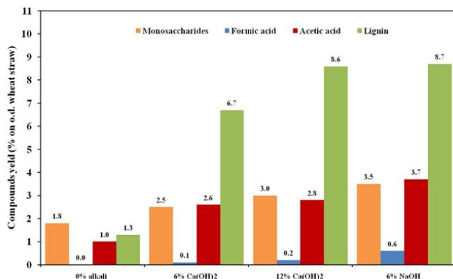
Fig. 5: Effect of NaOH and  $\text{Ca}(\text{OH})_2$  loading in extrusion pretreatment of wheat straw on yield of monosaccharides, formic acid, acetic acid and lignin in filtrates.
