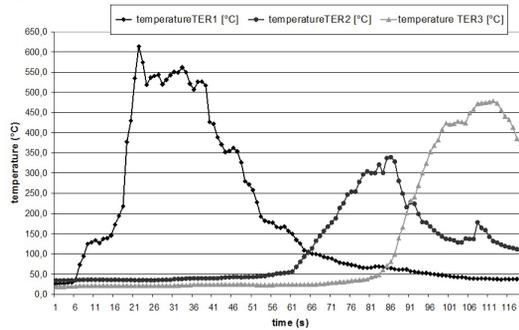
Fig. 3: Temperature curves for the  $0.5 \text{ m}\cdot\text{s}^{-1}$  measurements.
