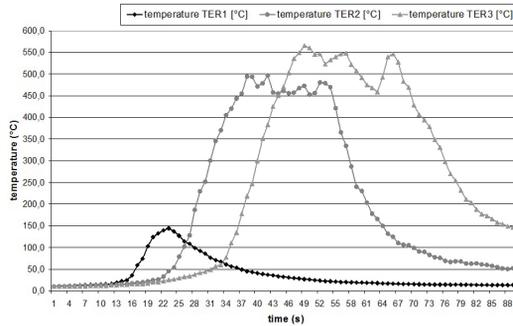
Fig. 5: Temperature curves for the 2.5 m.s<sup>-1</sup> measurements.
