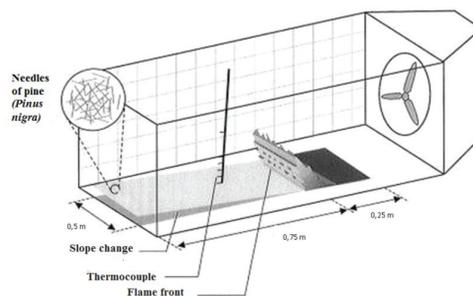
Fig. 1: Scheme of wind tunnel with a description of the individual parts.
