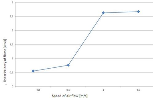
Fig. 7. Plot of linear velocity of flame spread for the selected air velocity within the model forest fire.
