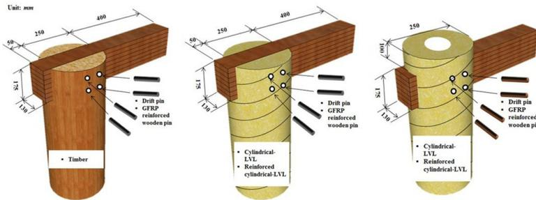
Fig. 4: Shape of moment resistance test specimens.
