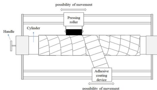
Fig. 2: Schematic diagram of spiral-winder.
