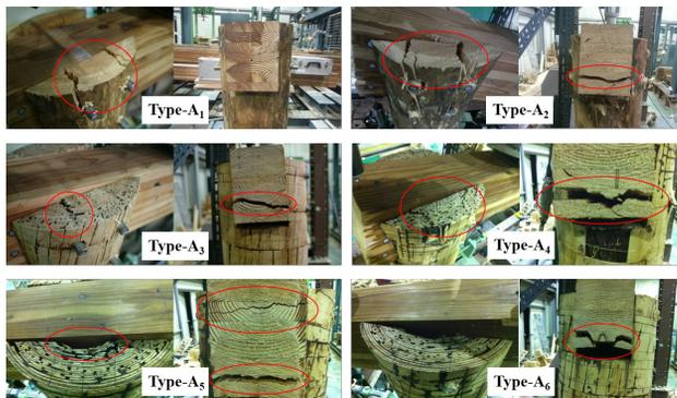
Fig.8: Failure modes of Type-A.
