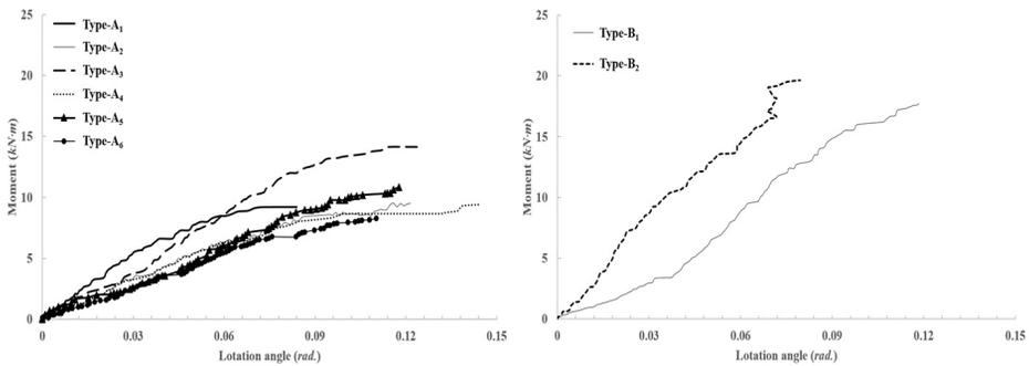
Fig. 7: Moment-rotation angle curves of moment resistance test.
