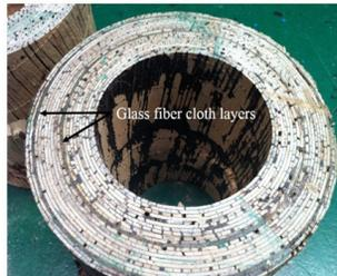
Fig. 3: Shape of cylindrical-LVL.
