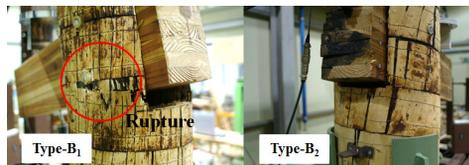
Fig. 9: Failure modes of Type-B.
