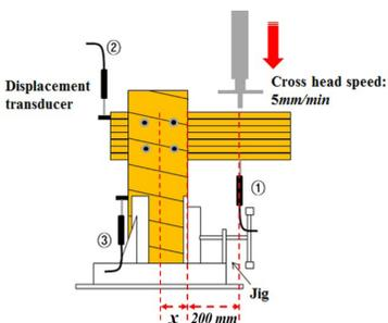
Fig. 5: Schematic diagram of moment resistance test.
