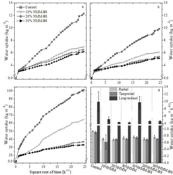
Fig. 5: Radial a), tangential b) and longitudinal c) water uptake (average of 20 samples) and the water uptake coefficient d) of untreated beech wood and wood treated with NMM resin respectively NMM-dye (BS) resin (10 %, 20 %, 30 %).
