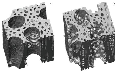
Fig. 6: Three-dimensional (3D) imaging of beech control a) size  $0.929 \mu\text{m}$  and of NMM-dye resin treated beech wood b) size  $1 \mu\text{m}$ .
