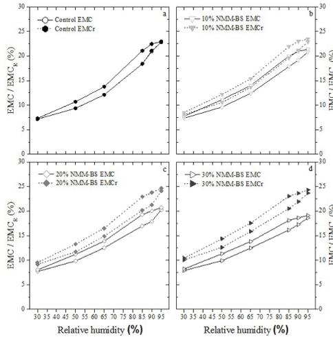
Fig. 2: Sorption isotherms of beech wood specimens; a): control, b): 10 % NMM-dye, c): 20 % NMM-dye, d): 30 % NMM-dye indicated as equilibrium moisture content (EMC) and reduced equilibrium moisture content ( $EMC_R$ ); 10 replicates were used per treatment.
