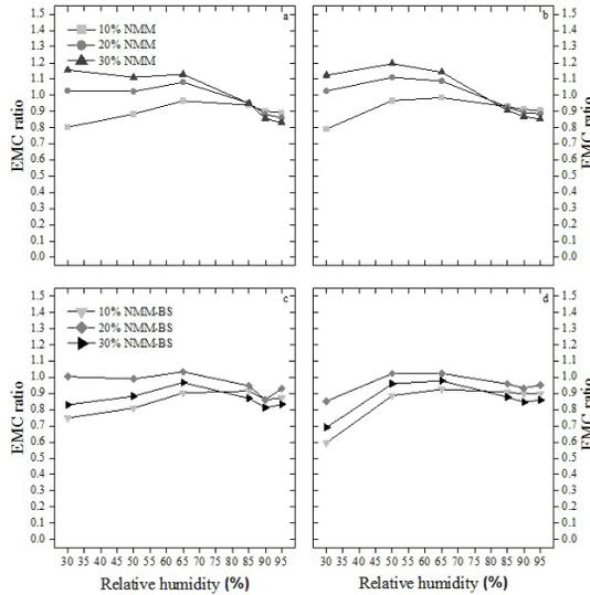
Fig. 3: EMC ratios of modified beech specimens ( $EMC_R$ ) related to their untreated control at adsorption (a, c) and desorption (b, d); 10 replicates were used per treatment.
