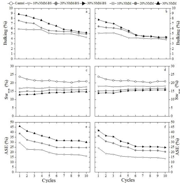
Fig. 1: Bulking (a, b), maximum swelling (b, c) and anti-swelling-efficiency [ASE] (e, f) of beech wood specimens treated to various WPGs with NMM resin (a, c, e) and NMM-dye resin (b, d, f) over 10 cycles of water saturation and oven drying; 10 replicates were used per treatment.
