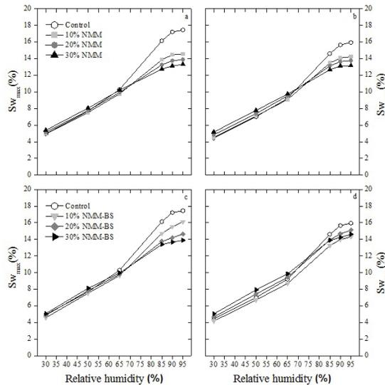
Fig. 4: Maximum swelling ( $Sw_{max}$ ) of beech wood modified with NMM (a, b) and NMM-dye (c, d) during moisture adsorption; a, c specimens without leaching, b, d after 10 cycles of leaching (EN 84, 1997); 10 replicates were used per treatment.
