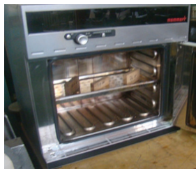
Fig. 1: Laboratory oven used for torrefaction process.
