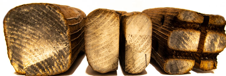
Fig. 6: The timber elements after the fire test.
