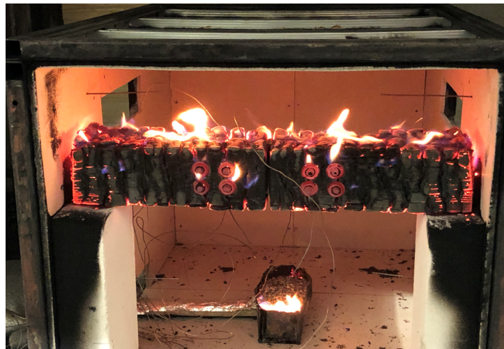
Fig. 4: Specimen 1 before taking out of the furnace and cooling down in the water.
