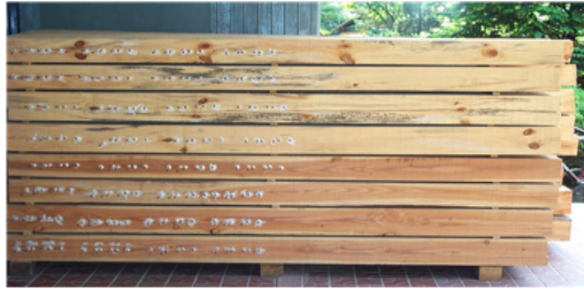
Fig. 1: Staking of timbers and nails inserted in stacking pile.
