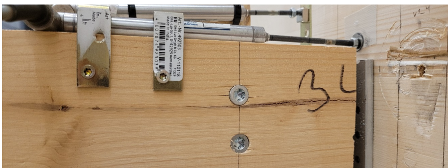
Fig. 7: Brittle failure of specimen 3, variant 2.
