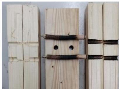
*Fig. 6: The failure mode of composites dowel.*
