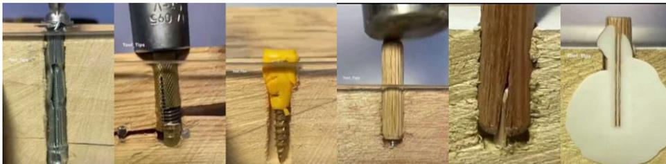
*Fig. 1: The disadvantages of the joints connected by wood dowels and self-tapping screws.*
