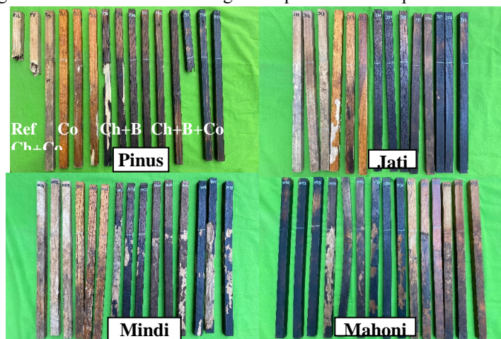
Fig. 5: Subterranean termite attack on wood samples after 12-week burial test.
