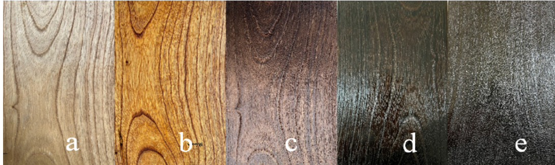
Fig. 1: Melia azedarach (mindy) samples: (a) untreated, (b) coating without charring, (c) charring and brushing (Ch+B), (d) charring, brushing and coating (Ch+B+Co), and (e) charring and coating (Ch+Co).
