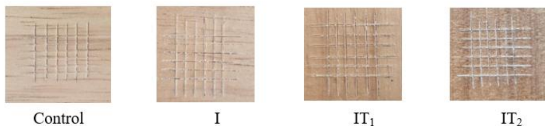
Fig. 7: Cross-cut lines of adhesion determination for control, surface-densified (I), densified and post heat-treated ( IT_1 , IT_2 ) rubberwood.
