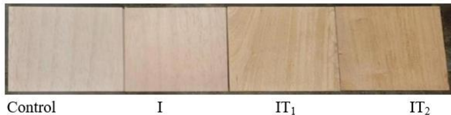
Fig. 4: Wood colour comparison of control, surface-densified (I), densified and post heat-treated (IT 1 , IT 2 ) rubberwood.
