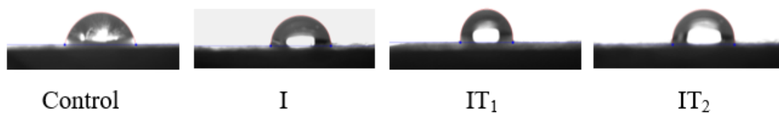
Fig. 5: The pictures of water contact angle of control, surface-densified (I), densified and post heat-treated ( IT_1 , IT_2 ) rubberwood.
