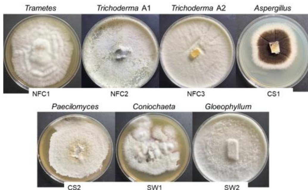
Fig. 1: Fungi isolates obtained, code keys meaning natural forest conditions (NFC1, NFC2 and NFC3), commercial sawmill (CS1 and CS2), in service structural wood (SW1 and SW2). Images taken 5 days after the fungus began to grow.
