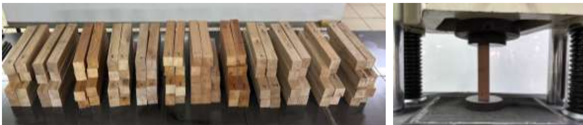
Fig. 1: a) Twelve tropical species of timber used in the research, b) compression test parallel to the grain according to ASTM D143-22.
