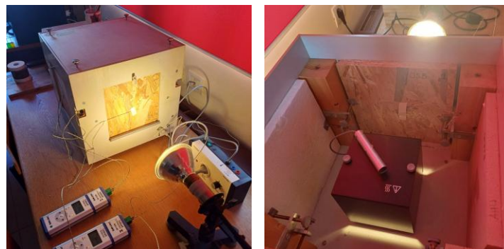
Fig. 1: PHYWE apparatus for measurement of thermal conductivity.
